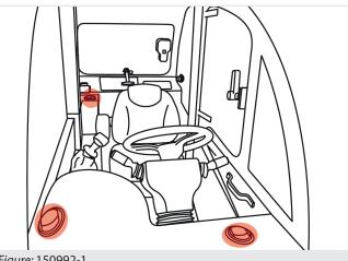
To open the air vents press on one side of these and adjust the air flow direction using the fins or rotating
