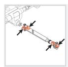
Drive shafts lubrication points.
