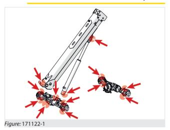
The automatic 5-point lubrication system lubricates the following points:
