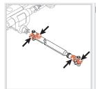
Drive shafts lubrication points.
