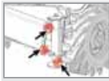
Outriggers lubrication points.
