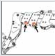
Boom with chains lubrication points.
