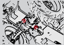
Swinging axle lubrication points.
