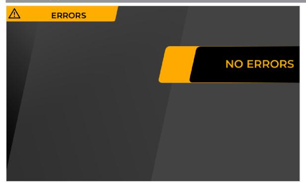
In the event of an error, the corresponding icon (A0), error code (A1a) and error description (A1b) are displayed on the Home page. In addition, an acoustic signal of 1.5 seconds is generated.
