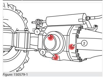
The filler, level and drain caps are located in the central part of the front and rear differential axle (fig. 150579-1):
