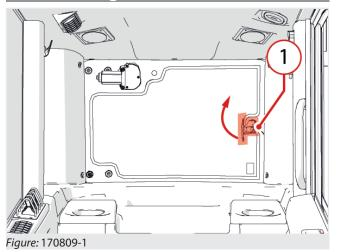
To open the rear glass, lift the handle "1" and push the glass outward.
