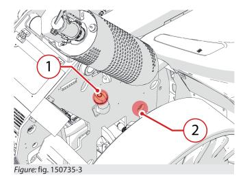
If necessary, remove the cap "1" (fig.150735-3) and add oil until it reaches the proper level.
