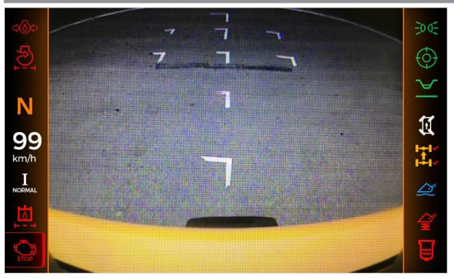
When reverse gear is engaged, an intermittent acoustic alarm will sound and the camera (if fitted) at the rear of the vehicle will turn on.
