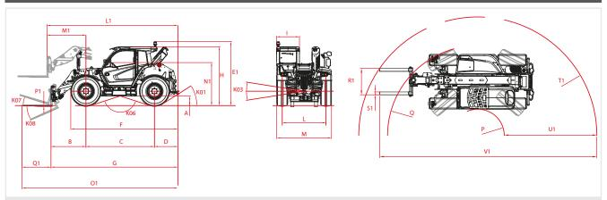
Figure: 180201-1: Dimensions with standard wheels
