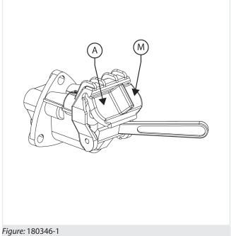
The pneumatic braking type CUNA has a single aluminum coupling:
