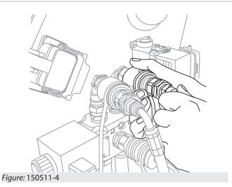
To connect the Push-Pull quick couplings to the valve on the boom head:
