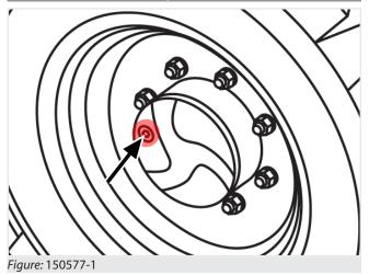
The oil cap of the epicycloidal reduction gear is located on the wheel hub (fig. 150577-1):
