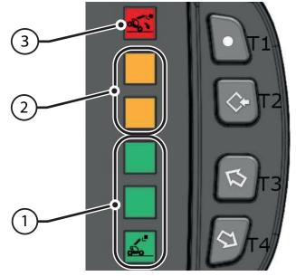
The longitudinal momentum indicator consists of a series of LEDs on the dashboard:
