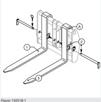
The data necessary for the identification of the forks are positioned on the right side of the forks, in the upper part "A" (fig. 150518-1).
