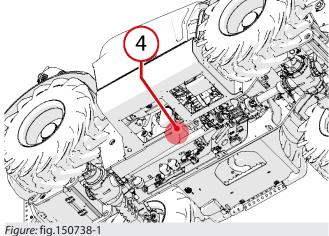
To replace the hydraulic oil filter (fig. 150738-1) carry out the following operations:
