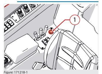
The USB sockets "1" (fig. 171218-1) allow to connect direct current devices (battery chargers, cell phones, etc.).
