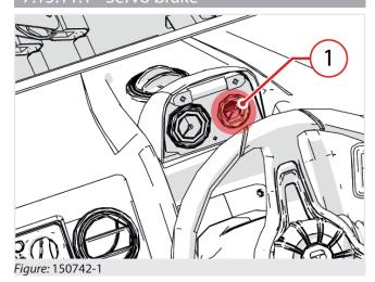
The pressure gauge "1" (fig. 150742-1) is used to control the servo brake pressure. In case of anomalies and faults, the pressure may drop.
