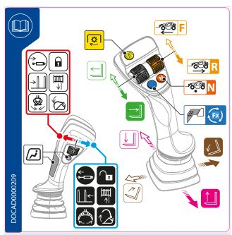
Figure: 180301-1: Instructions for using the joystick
