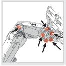
Counter lever and swing cylinder lubrication points.
