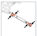
Drive shafts lubrication points.
