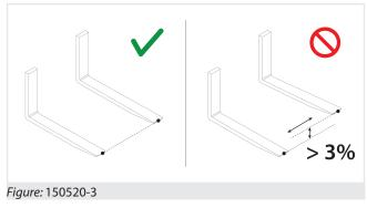
For example, for a fork 1800 mm long, the difference between the maximum permissible deformation of the fork tips will therefore be of 54 mm (1800 x 3/100 = 54).
