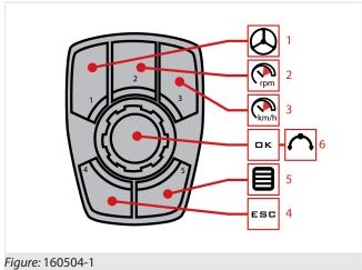
The Maximum speed limiter selection key "3" (fig. 160504-1) is used to set the vehicle movement maximum speed.
