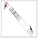
Lifting cylinder lubrication points.
