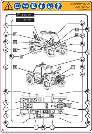
Figure: Most frequent maintenance operations
