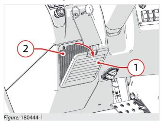
To replace the internal air filter in the cab, it is necessary to (fig. 180444-1):
