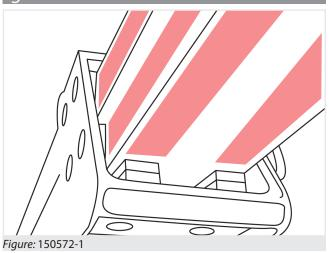
The boom sliding blocks must be kept lubricated to prevent as much as possible the deterioration and maintain soft movements.
