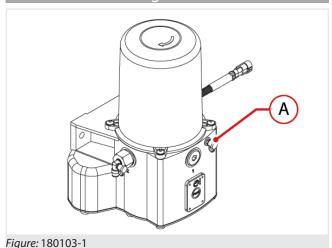
The pump tank is filled using the lubricator "A".
