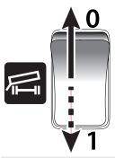
Figure: Pressure relief switch
