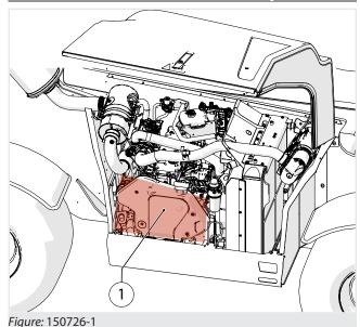
Check that the belt "1" (fig. 150726-1) does not have cuts, cracks or rubbing signs; when in doubt, install a new belt.
