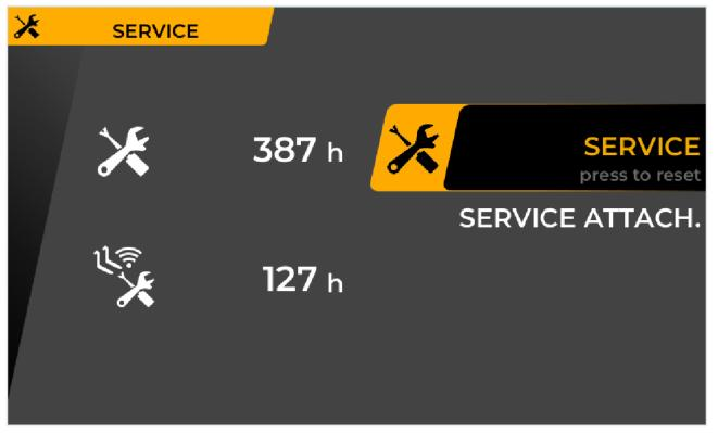
This page displays the countdown of the vehicle service hours and the countdown of the service hours of the accessories.
