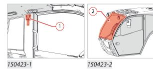
The front glass of the cab (fig. 150423-1) can be used as an emergency exit in case the vehicle doors are locked.
