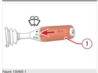
Press the middle button on the lever "1" (fig. 150405-1) to turn on the front window washer.
