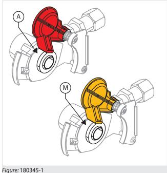
The pneumatic braking of EEC type includes two couplings:
