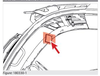
Adjust the internal rear-view mirror (fig. 180330-1) to have a good rear view during long trips.
