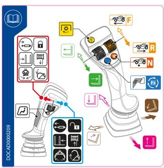
Figure: 180301-1: Instructions for using the joystick
