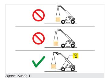
To keep the suspended load from swaying while being handled, the load can be fixed to the anchoring eyebolts of the vehicle while being transported.
