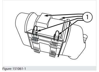
An air filter (fig. 151061-1) in bad conditions results in the reduction of power, excessive fuel consumption and reduced engine life.
