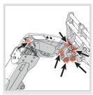
Counter lever and swing cylinder lubrication points.
