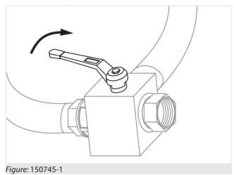
DANGER! When rotating the handle a jet of oil under pressure may leak out from the valve. Use appropriate safety equipment to protect eyes and skin from hot oil under pressure.
