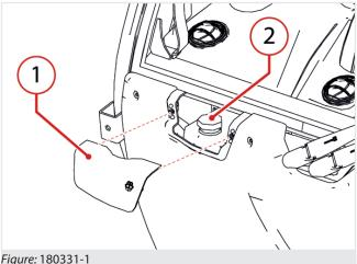
The washer fluid tank is located on the front external side of the cab (fig. 180331-1).
