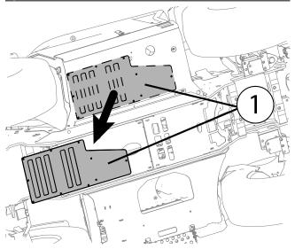
To perform maintenance operations it is necessary to temporarily remove the under chassis protection of the vehicle. The under chassis protection protects the bottom of the vehicle, from any bumps, collisions, dirt.
