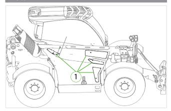
Check that the air recirculation grids and nets are clean and free from dirt:
