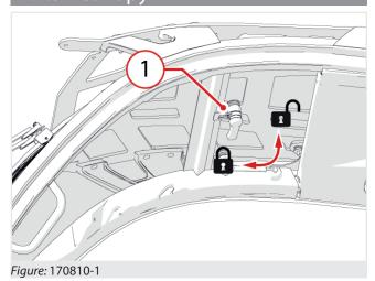
To open the roof, turn the handle "1" (Fig. 170810-1) to the open position and raise the roof.
