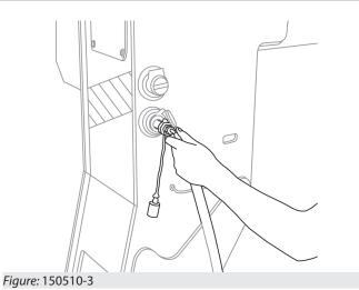
To connect the Push-Pull quick couplings to the sockets on the boom head:
