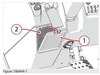
To replace the internal air filter in the cab, it is necessary to (fig. 180444-1):
