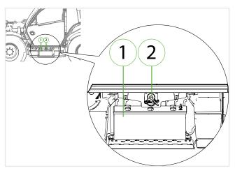
The battery isolation switch "2" (150731-1) allows the operator to isolate the battery "1" from the electrical circuit in case of emergency or during maintenance operations.
