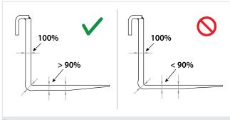
For example for a fork 70 mm thick, the thickness must not be less than 63 mm. (70 - 10% = 63)
