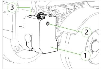
The hydraulic oil tank "1" is located on the rear side of the vehicle, in the central part.
