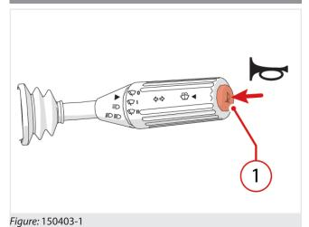
Press the button on the end of the lever "1" (fig. 150403-1), to activate the horn.
