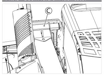
14.9.4 - Lifting cylinder lubricators
