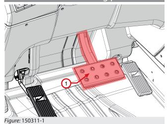
Press the service brake pedal "1" (fig. 150311-1) to slow down or stop the vehicle.
