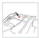
Boom-chassis pin lubrication points.
