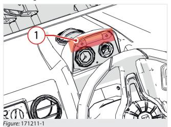
To safely operate, the spirit level must be at the centre, with a maximum approximation of 2° to the right or left.
