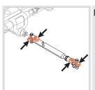
Drive shafts lubrication points.
