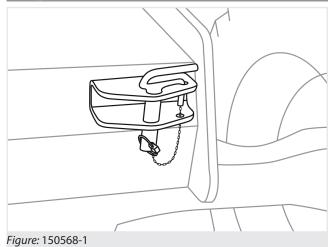
In case it is necessary to tow the machine with engine in failure, follow the following steps:
