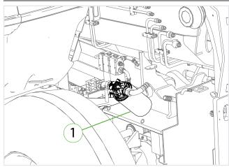
To replace the hydraulic oil filter carry out the following operations:
