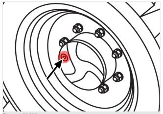
The oil cap of the epicycloidal reduction gear is located on the wheel hub (fig. 150577-1):
