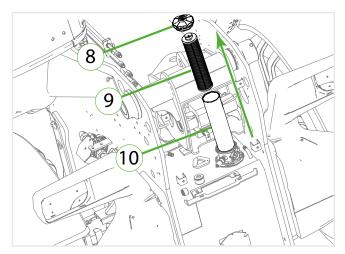
The hydraulic oil return filter is located inside the hydraulic oil tank.
