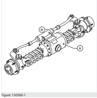
The parking brake must be disengaged directly on the front axle with the engine off to allow the vehicle to
