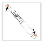
Lifting cylinder lubrication points.
