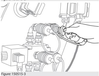
To disconnect the Push-Pull quick couplings from the valve on the boom head:
