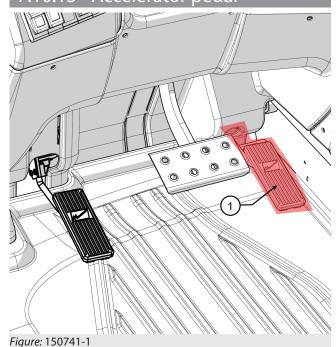
Press the accelerator pedal "1" (fig. 150741-1) to increase the engine speed, when the pedal is released the engine rpm will decrease.
