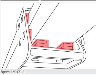
Worn sliding blocks can lead to oscillations and clearances between one extension and the other with consequent loss of precision in the movements and danger of load falling.
