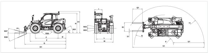
Figure: Dimensions with standard wheels
