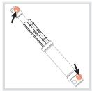
Lifting cylinder lubrication points.
