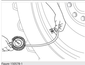
Verify and adjust the pressure of the front and rear tires.
