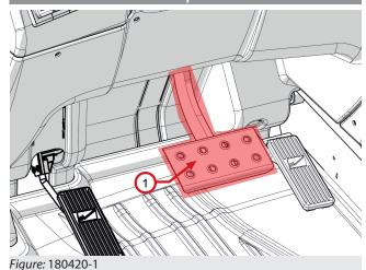
Visually check that the joints of the pedals (fig. 180420-1) are not damaged and that the pedal stroke is not excessive or too elastic.
