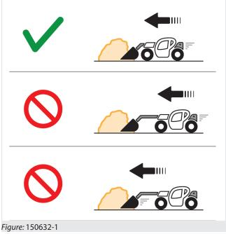
It is strictly forbidden to push or stack material with the vertical bucket planted in the ground.
