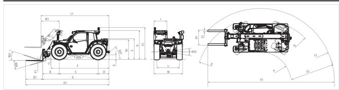
Figure: 180201-1: Dimensions with standard wheels
