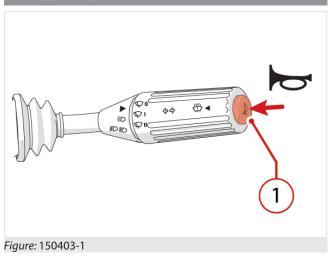
Press the button on the end of the lever "1" (fig. 150403-1), to activate the horn.
