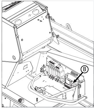
Figure: Wired control connection on the vehicle
