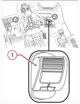
In emergency conditions, if the brake does not work, the machine can be stopped by means of the unstable emergency stop lever "1" located in the cab. Keep the lever pressed downward to let the machine be stopped smoothly.
