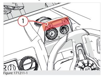
To safely operate the spirit level must in the center, with a maximum approximation of 2° to the right or left.
