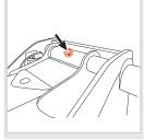
Boom-chassis pin lubrication points.
