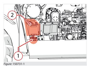
The battery isolation switch "1" (150731-1) allows the operator to isolate the battery from the electrical circuit in case of emergency or during maintenance operations.
