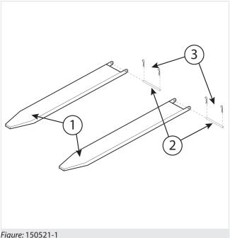
The fork extensions consists of the following main components (fig. 150521-1):
