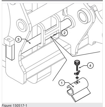
The Forks block prevents lateral movement of the forks once the desired setting has been chosen.
