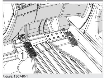
The inching pedal "1" (fig. 150740-1) acts directly on the hydrostatic transmission and allows to slow down the vehicle forward movement.
