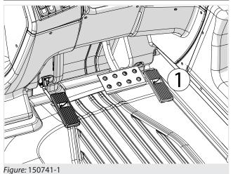
Press the accelerator pedal "1" (fig. 150741-1) to increase the engine speed, when the pedal is released
