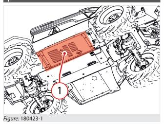
To perform maintenance operations it is necessary to temporarily remove the under chassis protection of the vehicle. The under chassis protection protects the bottom of the vehicle, from any bumps, collisions, dirt.
