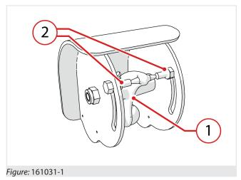
The bucket position is determined according to the position of the pendulum "1" compared to the indicators "2":
