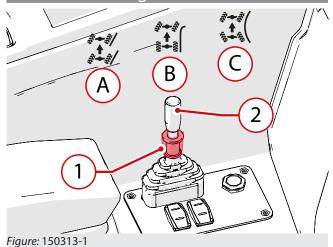
The steering selector lever (fig.150313-1) is used to change the steering mode of the wheels:
