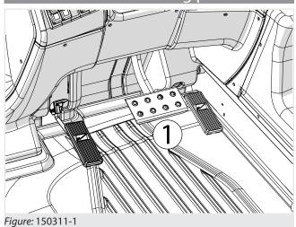
Press the service brake pedal "1" (fig. 150311-1) to slow down or stop the vehicle.
