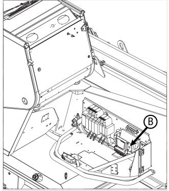
Figure: Wired control connection on the vehicle
