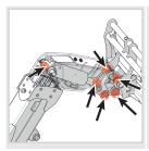
Counter lever and swing cylinder lubrication points.
