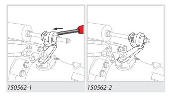
The parking brake must be disengaged directly on the axle to allow the vehicle to be towed.
