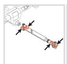
Drive shafts lubrication points.
