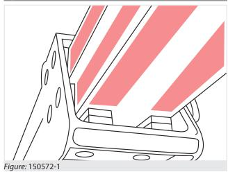
The boom sliding blocks must be kept lubricated to prevent as much as possible the deterioration and maintain soft movements.
