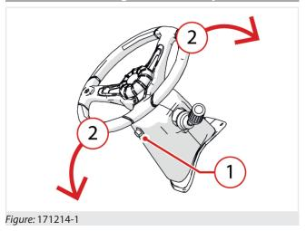
To adjust the steering wheel tilt (fig. 171214-1):
