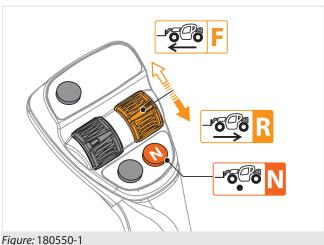
On the Joystick there is the F/R roller that is used to select the direction of travel in a faster and more ergonomic way:
