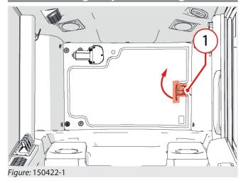
The rear glass of the cab (fig. 150422-1) can be used as an emergency exit in case the vehicle doors are locked.
