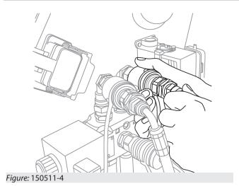
To connect the Push-Pull quick couplings to the valve on the boom head:
