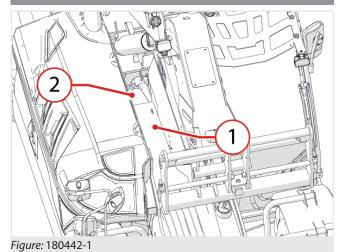
To replace the hydraulic oil filter (fig. 180442-1) carry out the following operations:
