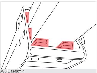
Worn sliding blocks can lead to oscillations and clearances between one extension and the other with consequent loss of precision in the movements and danger of load falling.
