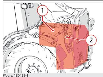
The hydraulic oil tank "1" (fig. 180433-1) is located on the rear side of the vehicle, in the central part.
