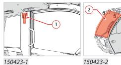
The front glass of the cab (fig. 150423-1) can be used as an emergency exit in case the vehicle doors are
