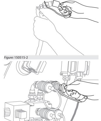
To disconnect the Push-Pull quick couplings from the valve on the boom head:
