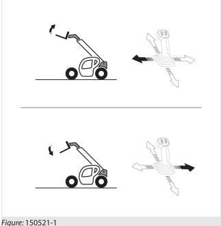
To use the forks it is sufficient to move the controls for the plate tilting.
