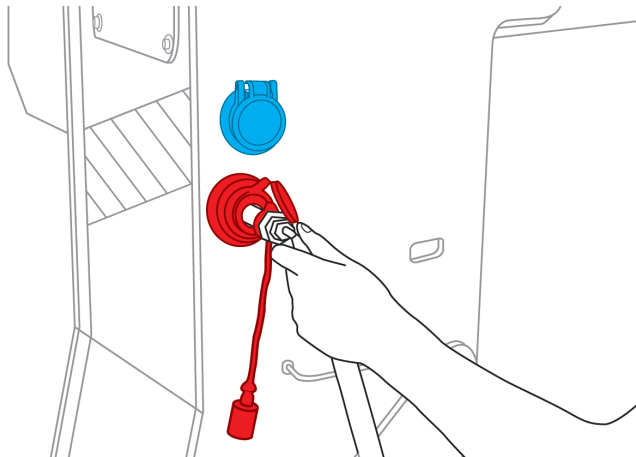
Figure: Hydraulic sockets on boom head
